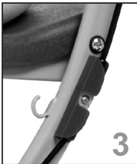
This photo shows how both cables appear when they have been properly secured in the anchor assembly. Note that the plastic-covered cable ends lock into the anchor assembly to keep the cable firmly in place during use.
